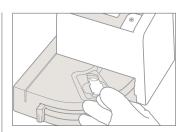
Place microcuvette into analyzer.
