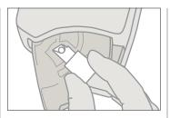
Place the microcuvette into the analyzer.
